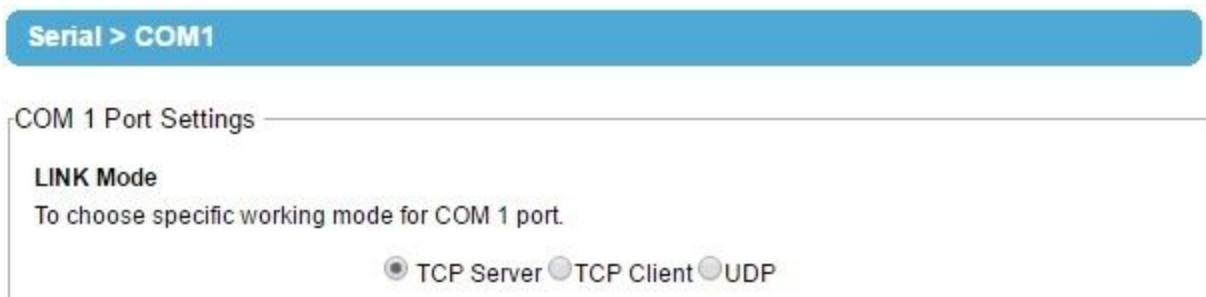
Figure 4.1 - Link Mode Options for COM1 Port
