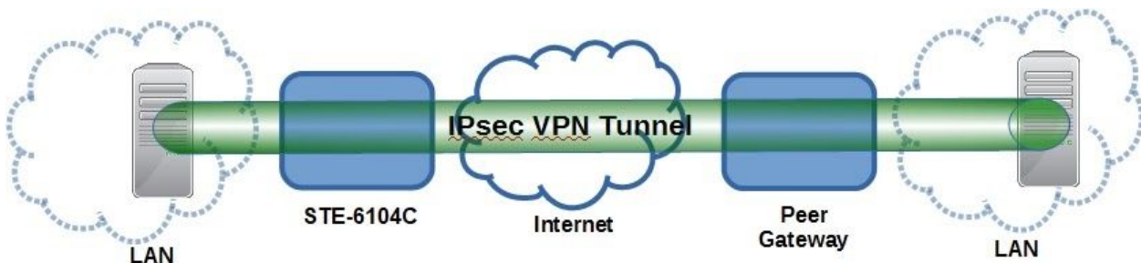
Figure 3.41 - An example of host-network application via the subnet-to-subnet connection
