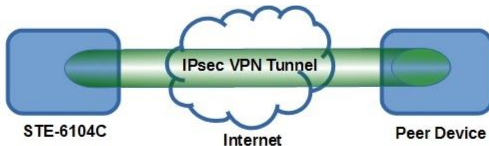
Figure 3.45 - IPsec VPN Tunnel with Host-to-Host Topology
