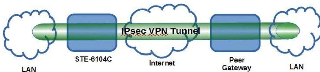
Figure 3.51 - IPsec VPN Tunnel with Network-to-Network Topology
