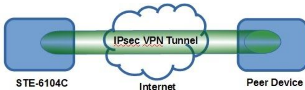
Figure 3.37 - An Example of a Host-to-Host Connection
